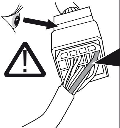
**(GB)** Please check if B+/30 permanent power wire in trailer preparation connector has got a minimum diameter of 1,5 mm<sup>2</sup>. If less than 1,5 mm<sup>2</sup>, continue with Option 2!
